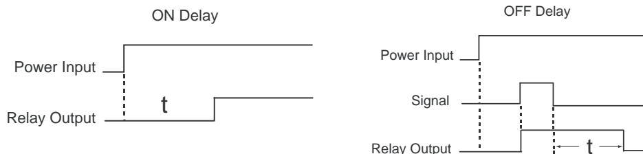
Figure 96 - Timing Diagrams for 700-HT Relays
